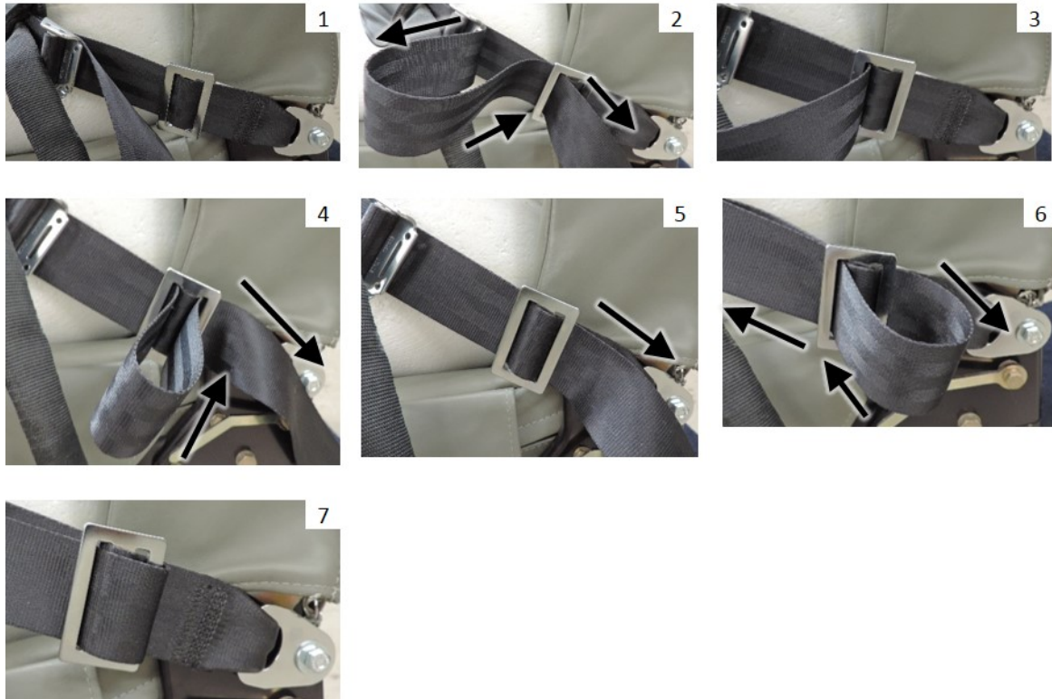
Figure 16. Threading Webbing Through the 3-Bar Slide
