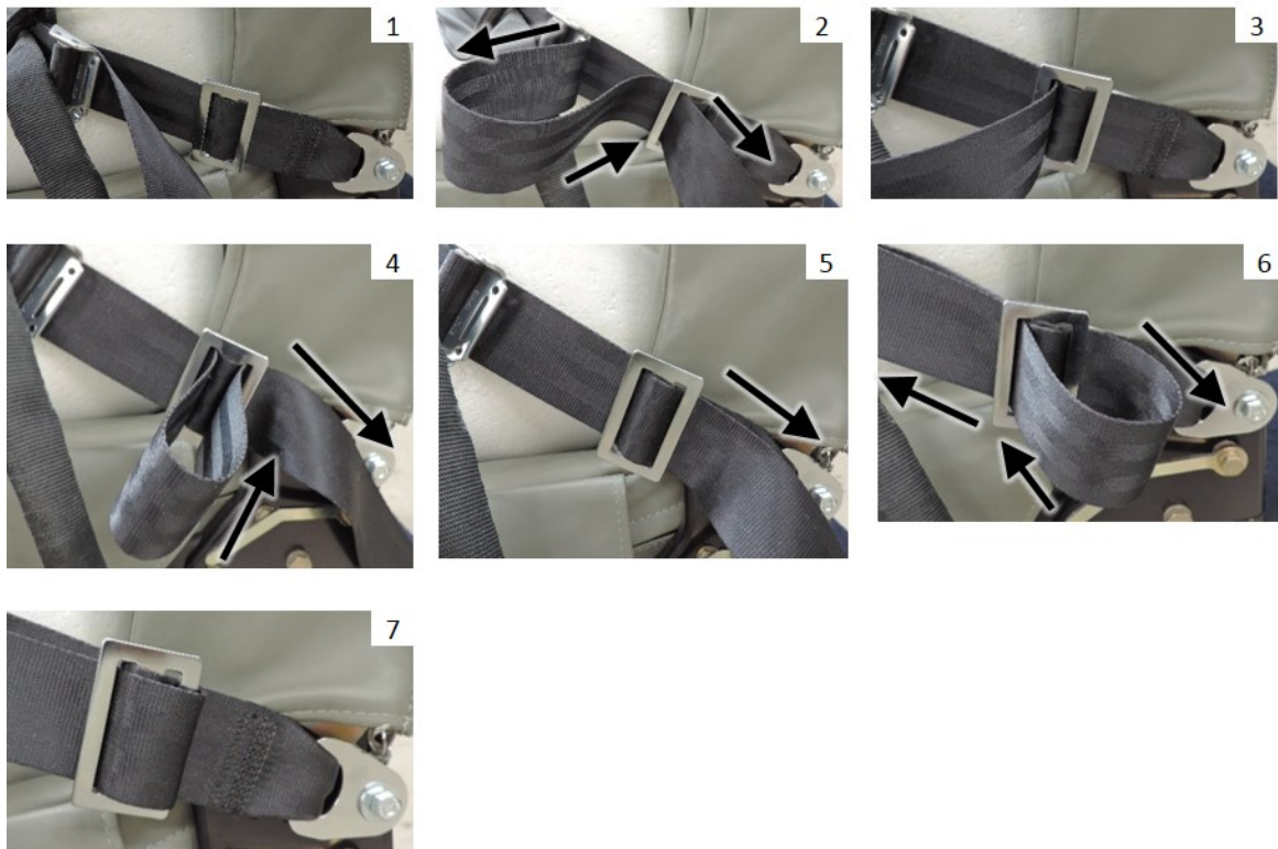
Figure 12017. Threading Webbing Through 3-Bar Slide (Graphic 25-10-01-99B-031)
