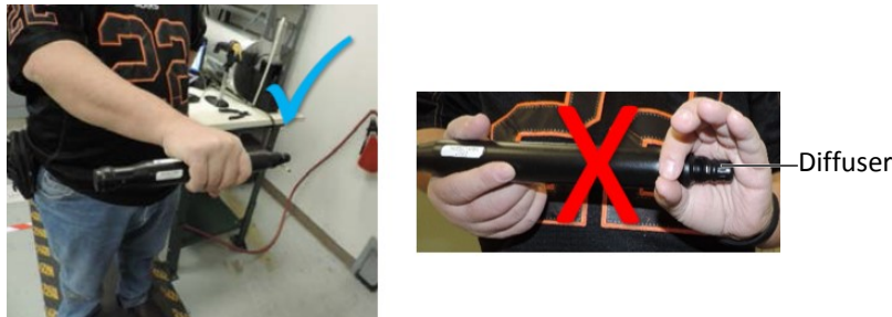
Figure 15002. Inflator Assembly Handling (Graphic 25-10-01-99B-048)
