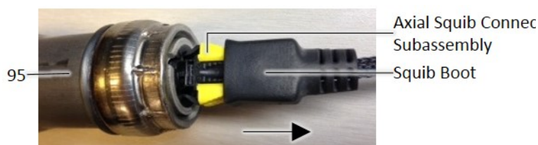
Figure 12004. Squib Connector Subassembly Connection to Inflator Assembly (95) (Graphic 25-10-01-99B-019)
