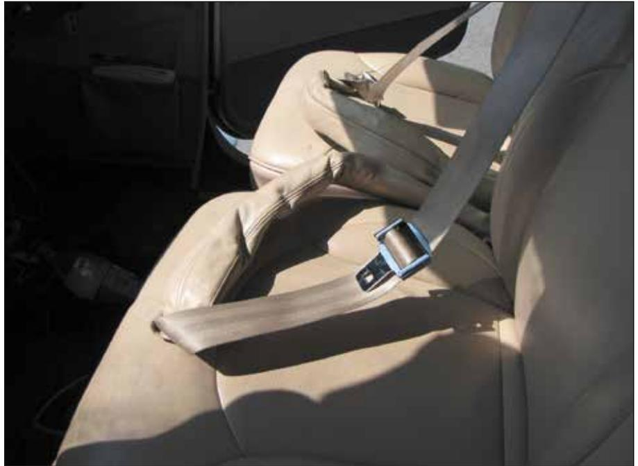
positioning provided by the belt and torso restraint an airbag system ranges from worthless to counterproductive—and protects against impact forces with an airbag specifically tailored for the shape of the space.
