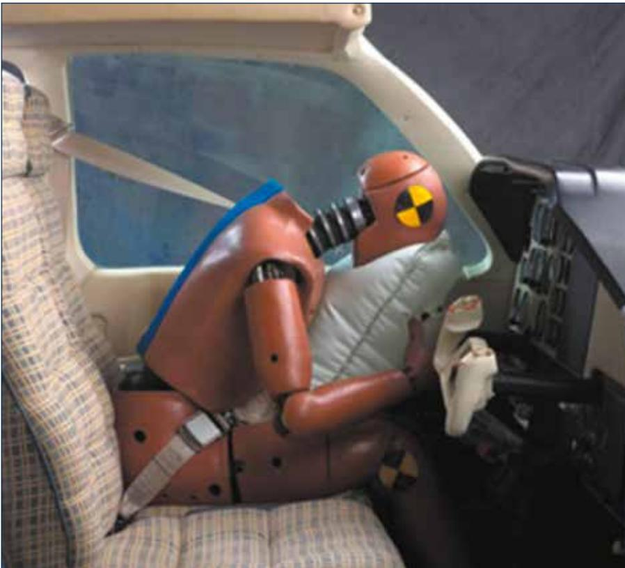
*In a three-point restraint system, the airbag is installed in the seatbelt, above right. For a four-point restraint, there is an airbag in each shoulder harness, below right.*
