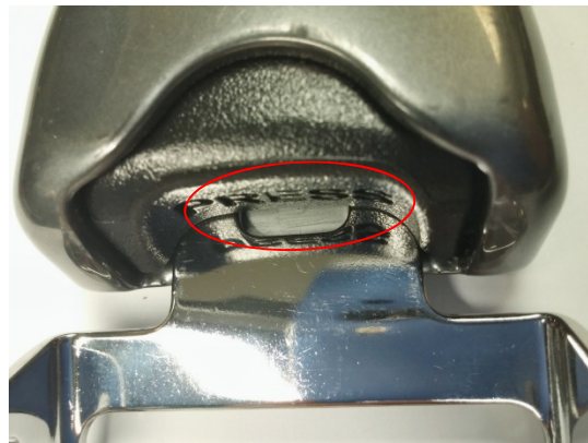
Figure 4: Connector not Fully Engaged
