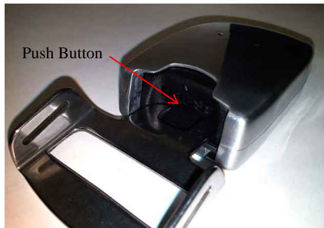
Figure 5: Push Button not Returning when Connector Inserted
