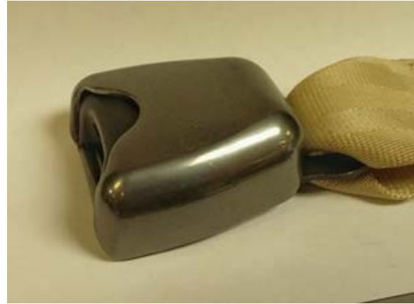
Figure 2: 505703-Series Buckle, Unaffected by Service Bulletin
