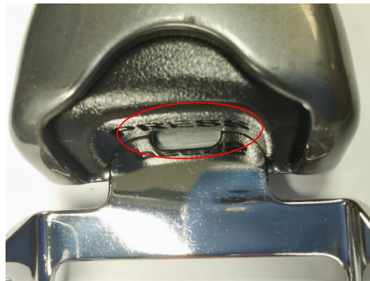
Figure 4: Connector not Fully Engaged
