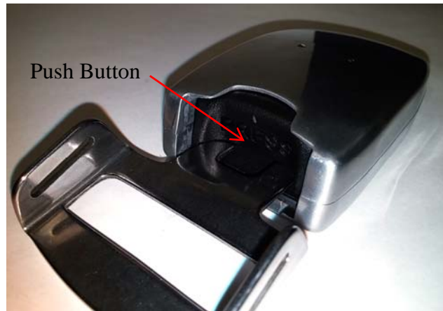
Figure 5: Push Button not Returning when Connector Inserted
